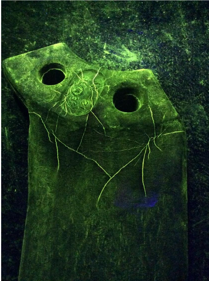
Figure W-2. Photograph of 4140 steel tine showing quench cracks after dye penetrant inspection.
