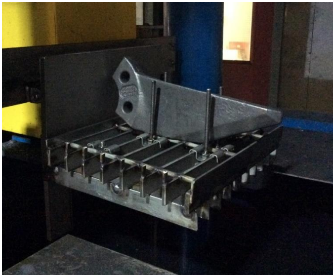
Figure W-1. Tine positioned on quench table showing the orientation of the part during the DFIQ process.
